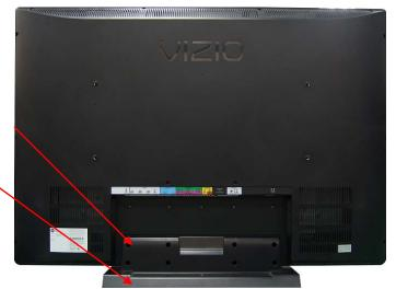
Note: The specs for these screws are self-tapping 4mm, 20mm long.
